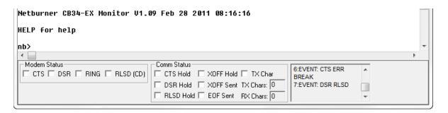
7. At the "nb>" prompt, type "setup" and press enter. You will now see what the current settings are for the IP Address, IP Mask, etc.
