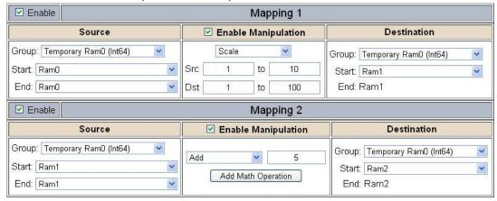
In this example, Ram0 is scaled into Ram1. Ram1 is then increased by 5 and stored into Ram2. Ram0 and Ram2 could be considered a source or destination group.
